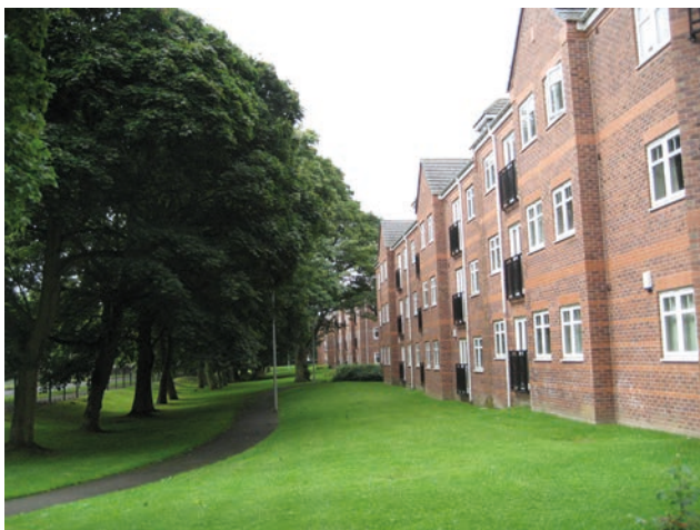
Good sustainable relationship: Sycamore trees to front SE. "A" distance is 12m (Guideline distance 10m). Location - Brackenhurst Drive LS17 6WE.
