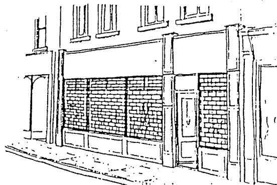
Fig.17 Both rigid demountable mesh panels and external mesh roller grilles are more obtrusive than internal grilles and so are less suited to sensitive locations such as Conservation Areas and on Listed Buildings.
