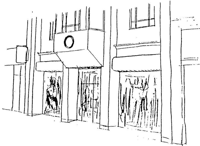
Fig.20 Fully glazed shop fronts can be vulnerable to ram raiding.
