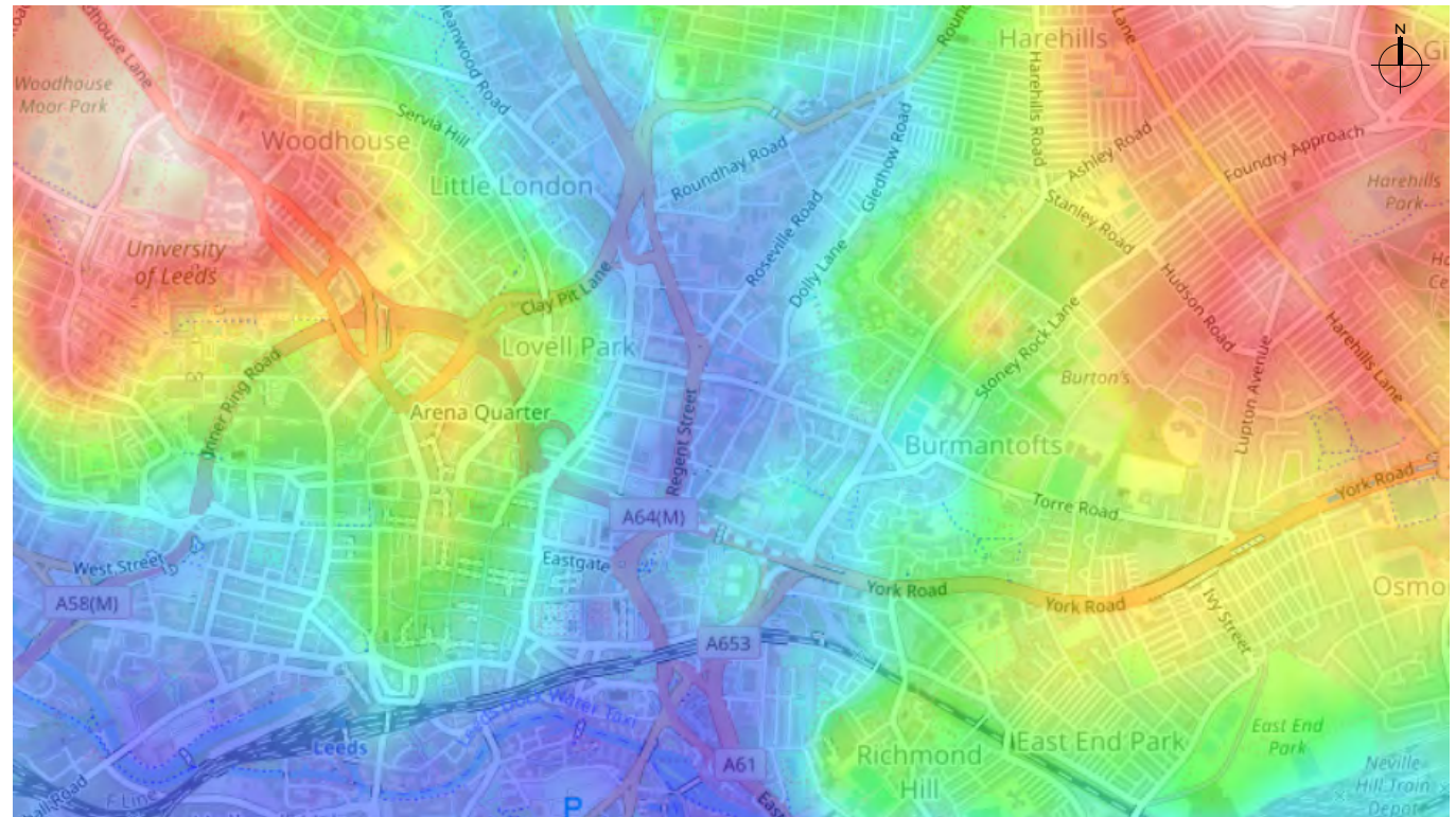
Topographic map of the area with Mabgate and Regent Street within the low lying valley (blue) containing the Mabgate Beck. The higher ground (green to red) lies to the east and west.
