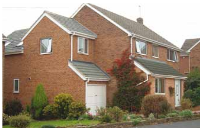
Care should be taken to ensure that windows are positioned to avoid overlooking neighbouring gardens.
